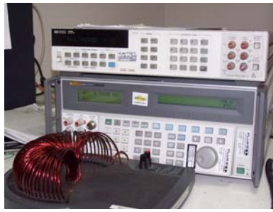
Electrical Calibration Workstation
