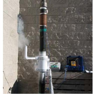
Electronic monitoring uses thermocouples installed in various locations at and near the ice plug to monitor the temperature. Visual monitoring uses colour/infrared cameras and remote monitors to observe the ice plug and frosting on the pipe.
